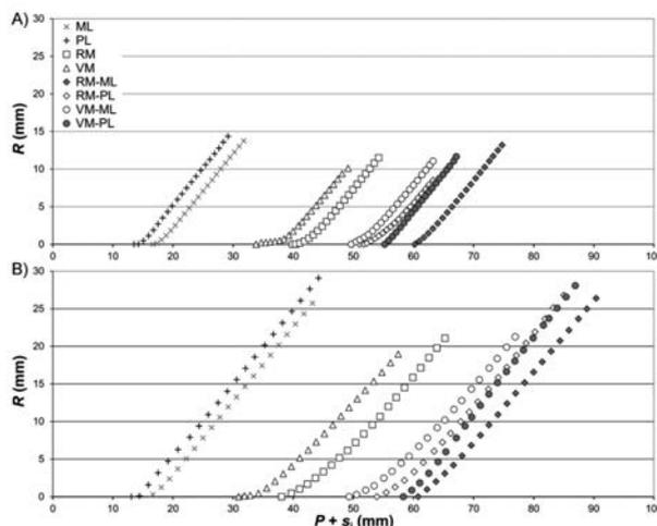
Figure 3. Drainage flux  $R$  versus the sum of the precipitation  $P$  and the initial water storage  $s_i$  (equal to  $WRC_{ob1}$ ) for the all tested samples. A) 2-years return period second storm; and B) 30-years return period second storm. ML, mineral layer; PL, preformed layer; RM, recycled medium; VM, volcanic medium.
