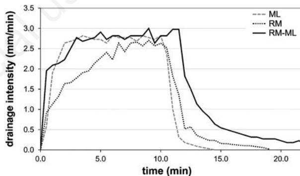
Figure 4. Drainage intensity collected during the tests on the mineral drainage/storage layer (ML), the growth media recycled medium (RM) and the green-roof samples RM-ML.
