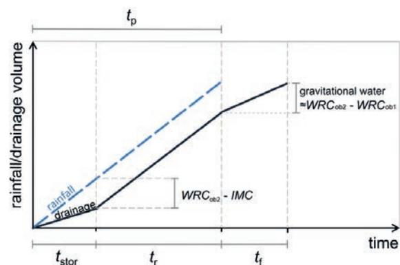
**Figure 6.** Schematic representation of the behaviour of a green roof with a given antecedent moisture content affected by high intensity rainfall;  $t_p$  is the precipitation duration,  $t_{stor}$  is the time required to reach  $WRC_{ob2}$  of the green roof,  $t_f$  is the delay between the conclusion of the storm and the time at which drainage stops flowing from the roof;  $IMC$  is the initial moisture content.
