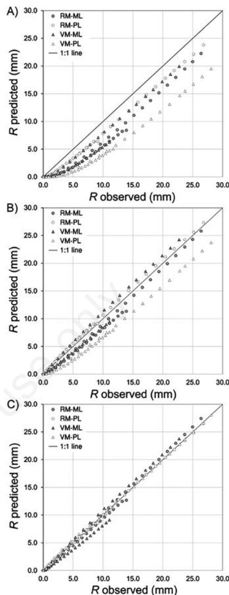
Figure 5. Comparison between the drainage observed in the laboratory and that predicted by A) the layers sequence model; B) the layers integration model; and C) the Curve Number method with the values of  $I_a$  and  $S$  directly calibrated on the whole green roofs (Table 2). RM, recycled medium; ML, mineral layer; PL, preformed layer; VM, volcanic medium.
