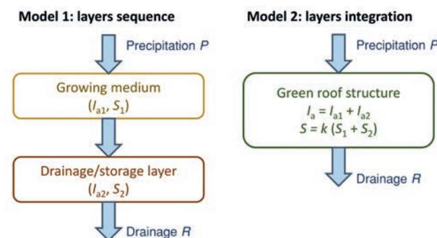
Figure 2. Graphical sketch displaying the structure of the two models used to apply the Curve Number method to green-roof structure starting from the hydrological proprieties of the single layers.
