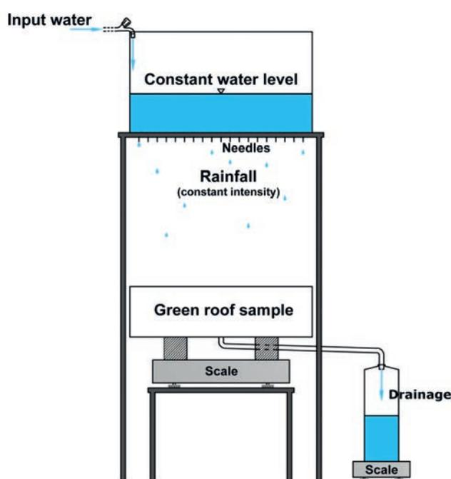
Figure 1. Schematic of the laboratory device.
